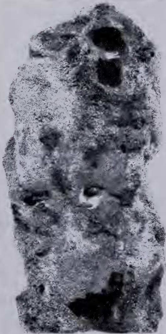
Figure 6.—Artificial fulgurite from Cottesloe. The light grey areas contain embedded sand grains, most of which have been altered to cristobalite. Length of specimen 19.5 cm.
